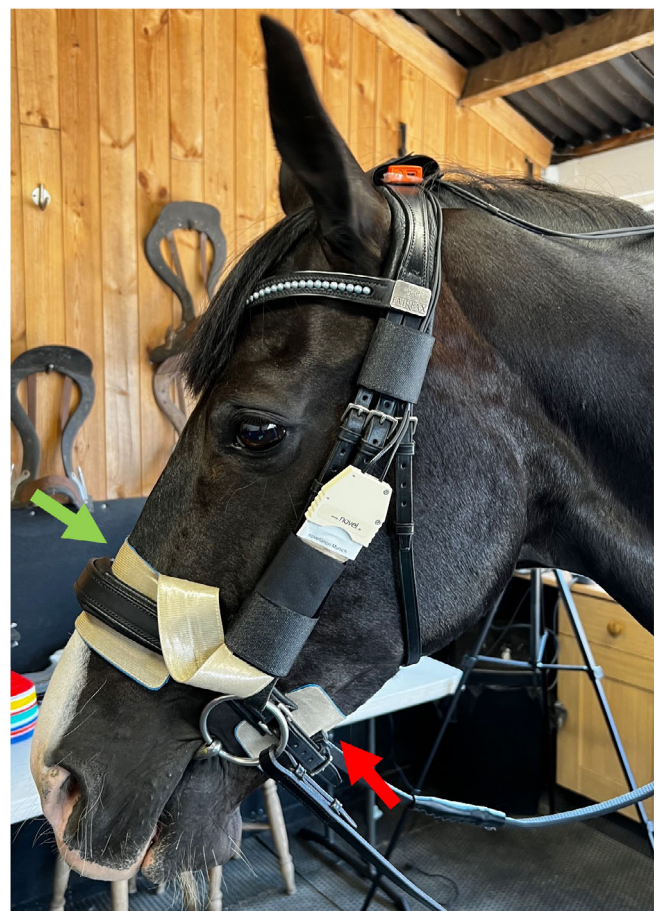
FIGURE 2 Positioning of the nasal (green arrow) and mandibular (red arrow) pressure mats beneath the noseband.
