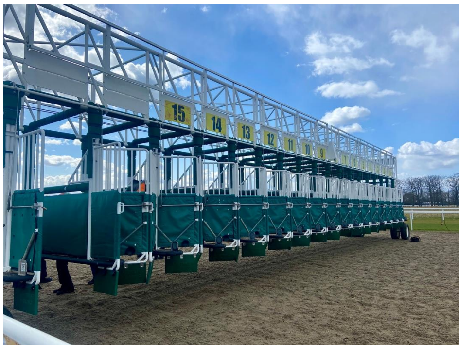
Figure 1: Starting stalls, also known as starting gates or barriers, are used to release horses simultaneously at the beginning of the race for a fair start. (Photo: Author IW's own)
